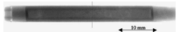
Fig. 4. X-ray image of capsule no. 8 (CuI) after irradiation in which a central region of lower density can be observed. The dotted line shows the position of the radial line scan, which is shown in Fig. 5.
